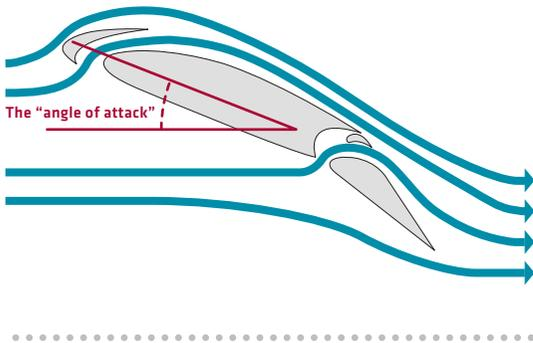
Spoilers up reduces lift and provides braking as the aircraft lands
