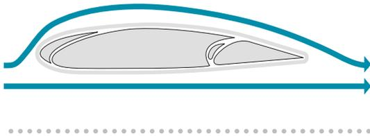
Extended with high angle-of-attack (the wing is angled towards the air flow)
