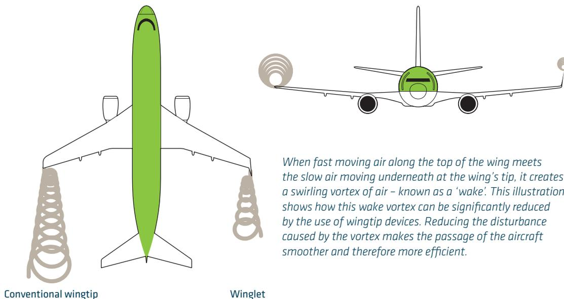
*When fast moving air along the top of the wing meets the slow air moving underneath at the wing's tip, it creates a swirling vortex of air - known as a 'wake'. This illustration shows how this wake vortex can be significantly reduced by the use of wingtip devices. Reducing the disturbance caused by the vortex makes the passage of the aircraft smoother and therefore more efficient.*
