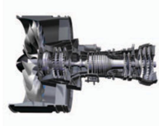
*A cutaway of the geared turbofan engine being developed by Pratt & Whitney*
